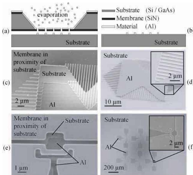
Figure 2: Illustration and SEM images showing the nanostencil deposition process. (a) 100-nm thick Al is evaporated from a distant source and deposited through the apertures in the membrane; (b) The stencil is removed from the substrate; (c) and (e) The SEM-images show the stencil mask and the underlying substrate; (d) and (f): The SEM-images show the resulting sub-micrometer Al structures.
