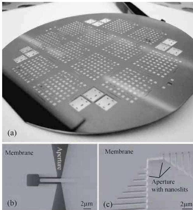
Figure 1: (a) Optical image of a 100-mm size full-wafer stencil containing various silicon nitride (SiN) membranes. The SiN layer is 200-nm thick. Each window contains numerous geometrical apertures as shown in the scanning electron micrograph (SEM) close-up of (b) and (c): Free-standing 200-nm thick SiN membrane containing micro and nano apertures ranging from 200 nm up to several 100  $\mu\text{m}$ .
