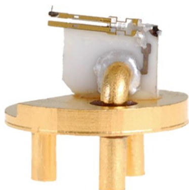
Figure 1: Image of a QPlus sensor mounted to the LT STM sensor carrier. Tungsten tips are glued onto the oscillating prong of the tuning fork. The use of W enables the QPlus sensor to be used simultaneously or alternatively in STM mode.
