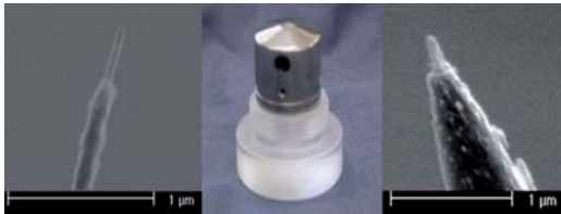
Fig.16: Left, electron micrograph of a single CNT grown on a tungsten tip. Note that the growth is aligned with the tungsten axis. Centre, a tungsten tip mounted in a suppressor module. Right, a CNT grown on a tungsten already mounted in the suppressor in situ.
