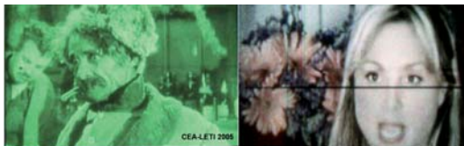
Fig.13: Two stages of development of CNT FED at CEA. On the left: monochrome display with 350\mu\text{m} pixels, on the right: color video display with 600\mu\text{m} pixels. On these display the non uniformity from pixel to pixel is 5% while it is 3% with LCD displays and 2% for CRT (courtesy of CEA-LITEN).
