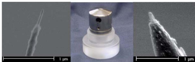
**Figure 10:** Left, electron micrograph of a single CNT grown on a tungsten tip. Note that the growth is aligned with the tungsten axis. Centre, a tungsten tip mounted in a suppressor module. Right, a CNT grown on a tungsten already mounted in the suppressor in situ.
