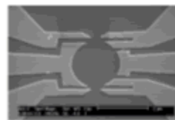
(Source: GaAs/AlGaAs heterostructure on top of which gates define a ballistic cavity. V.F. Bayo, CERN UCL)
