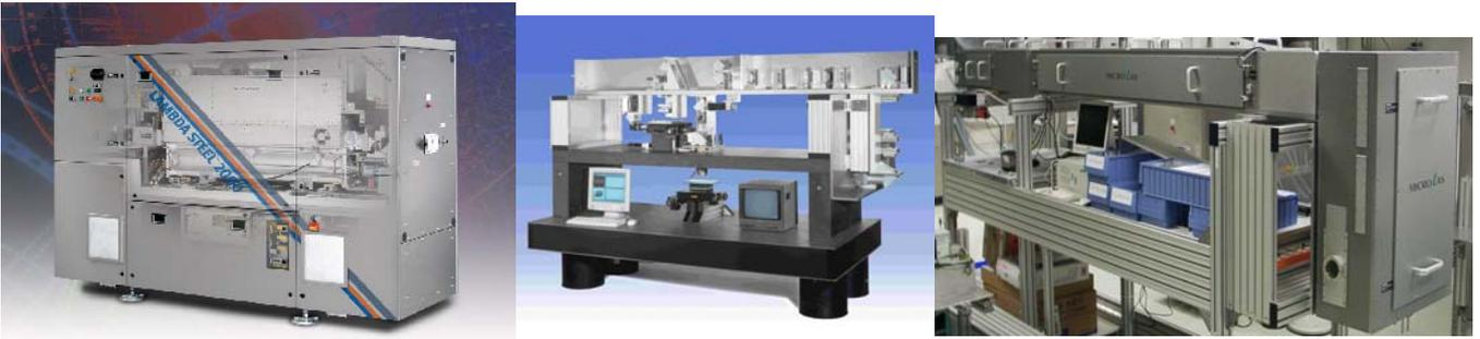
Laser and optics tools used in the project for irradiation of MOSFET wafers
