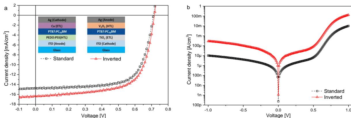
Figure 1 Current density – voltage characteristics under a) illumination AM 1.5G spectrum and b) darkness of both structures manufactured.
