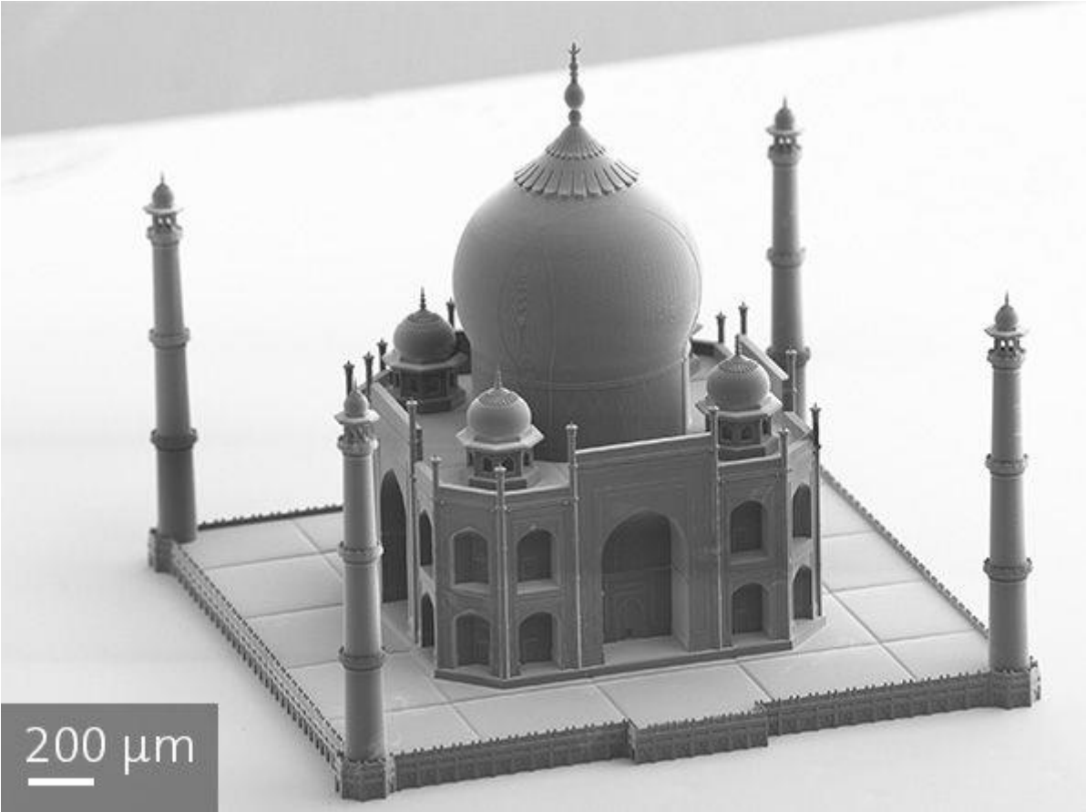
Fig 1: SEM image of the Taj Mahal demonstrating the fine features enabled by Nanoscribe's high-resolution 3D microprinting.
