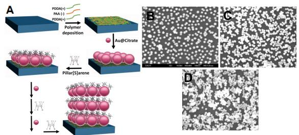
**Figure 1:** a) Schematic representation of the synthetic route where Au nanoparticles are deposited through electrostatic interactions in a multistep process. b-d) SEM images of the plasmonic substrate with 1, b); 2, c) or 3, d) additions of Au nanoparticles
