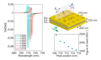
Left: TMOKE signal as a function of wavelength for varying values of the environment refractive index. Top-right: sketch of the structure used for the study. Bottom-right: figure of merit of obtained from the TMOKE curves.
