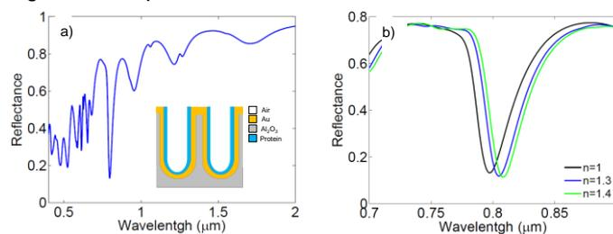
Figure 2: Study of sensing with a gold-coated NAA film.
