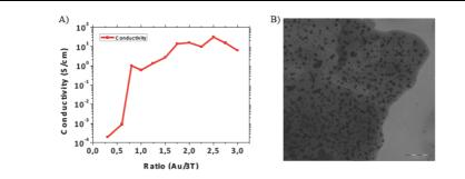
Figure 2: A) Dependency of IPN conductivity on Au/3T molar ratio. B) TEM image of the nanocomposite
