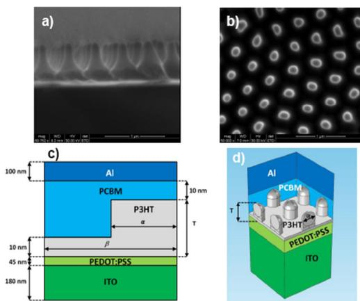
**Figure 1:** Environmental scanning electron microscopy (ESEM) images of P3HT nanopillars with the structure glass/ITO/PEDOT:PSS/P3HT-pillars made with NAAT, a) cross section and b) top view. Schematic unit cell (periodic conditions) of the structure ITO/PEDOT:PSS/P3HT/PCBM/Al for c) the 2D and d) the 3D models.
