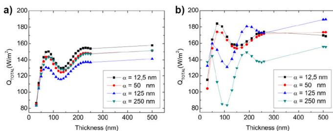
**Figure 2:** Total absorbed light power ( $Q_{TOTAL}$ ) in the P3HT layer of a) the 2D and b) the 3D models as a function of the nanopillars height ( $T$ ) for several nanopillar diameters ( $\alpha$ ).
