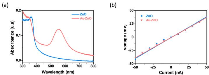
**Figure 2:** Optical and electrical characterization. a) UV-Vis spectra and of b) V-I Curve of ZnO and Au-ZnO films.
