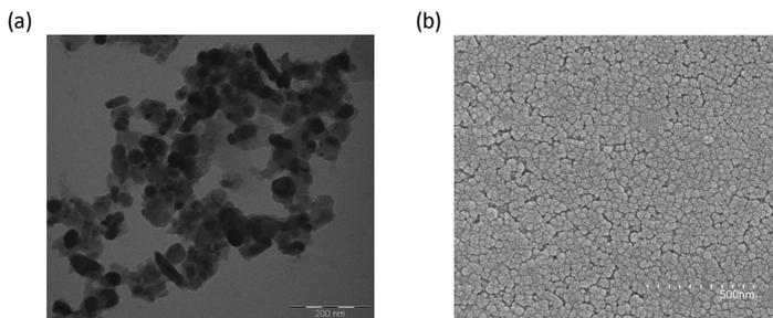
**Figure 3:** TEM (a) and SEM (b) images of Au-ZnO nanocomposite thin film.
