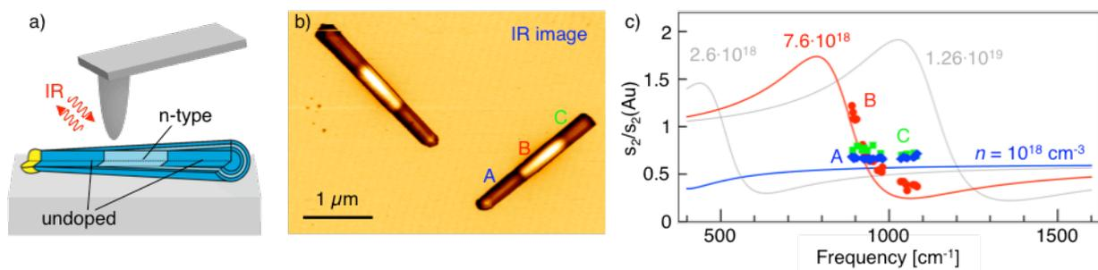
**Figure 1:** Infrared near-field mapping of modulation doped InP nanowires. (a) Schematic illustration of free-carrier profiling of modulation-doped semiconductor nanowires by infrared (IR) s-SNOM. (b) Amplitude  $s_2$  image of two representative InP nanowires recorded at an IR laser frequency of  $893 \text{ cm}^{-1}$ . (c) Experimental (symbols) and calculated (solid lines) local IR near-field amplitude spectra along a single InP nanowire.
