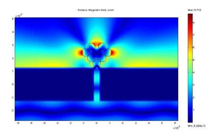
Magnetic field modulus (A/m) in a bifurcation with not vertical elbow (angle between chains at bifurcation: 90°, elbow angle: 90°. Distance between cylinders: 0*nm*) of seven metallic cylinders (refractive index n = 0.234+i1.275, radius r = 60nm) in front of a metallic slit (refractive index n = 0.135+i10.275, slab width: 2562.96*nm*, slab thickness: 258.13*nm*, slit width: 43.02*nm*) under p-polarization, wavelength: 346*nm*). The *LSP*11 mode is excited.
