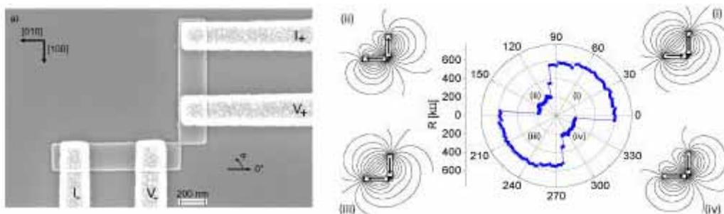
The field lines are very different depending on whether the magnetization of the two bars point towards each other (head-head) or one runs into the other (head-tail). The device can thus be written into one of the states illustrated in the schematics by applying a magnetic field in the proper direction, and then, after reducing the field to zero, be read out non perturbatively by measuring the constriction resistance. The device thus constitutes a non-volatile memory element.
