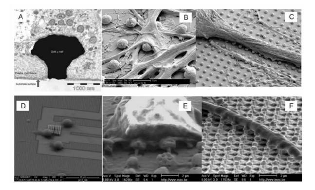
Experimental results: (A) transmission electron micrograph of a micronail engulfed by an Aplysia neuron (HUJI); (B) and (C) scanning electron micrographs of Aplysia neurons cultured on micronails (HUJI); (D) PC12 cells on a multielectrode chip with CMOS compatible (sub)micronails; (E) and (F) scanning electron micrographs of neuroblastoma cells (N2A) cultured on substrates with CMOS compatible (sub)micronails.
