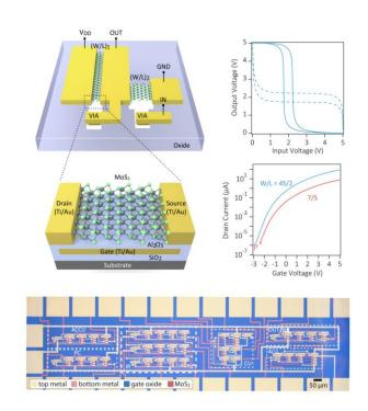
Figure 1: Schematic of an inverter circuit and an individual MoS<sub>2</sub>-transistor in gate-first technology (left) and measurement results of single transistors as well as inverters (right). The bottom shows an optical image of our microprocessor. testing, pads are used for Metal communications periphery and with wire-bonded together to realize internal connections.
