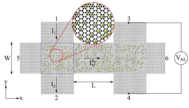
**Figure 1:** Schematic view of a six-terminal graphene device with gold adatoms
