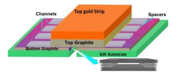
**Figure 1:** Schematic of the nanochannel device utilized for ion transport study. The width of the channel is 130 nm and the height can be varied from 1 atomic layer to several layers.
