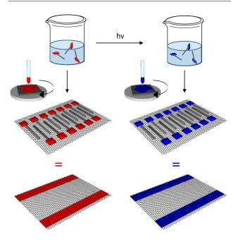
**Figure 1:** Cartoon of our approach for the formation of optically-tunable periodic potentials in hybrid organic/inorganic heterostructures.
