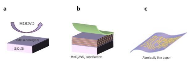
**a**, Schematics of wafer-scale uniform growth of TMD monolayers using MOCVD **b**, schematics of artificial stacking **c**, schematics of substrate free, atomically thin, and semiconducting paper
