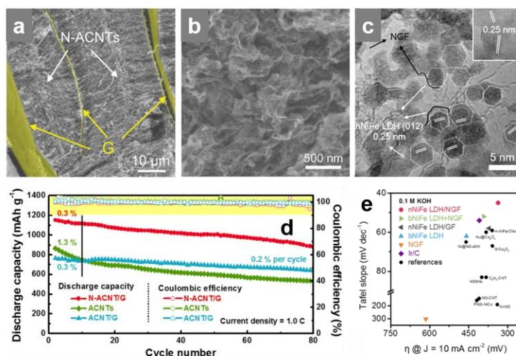
**Figure 1.** SEM image of a) N-ACNT/G and b) CaO-G, and c) TEM image of nNiFe LDH/NGF material. d) Li-S battery performances of N-ACNT/G and e) OER performances of nNiFe LDH/NGF.
