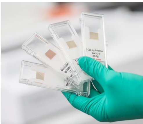
Figure 1. Biosensor chips based on monolayer graphene, graphene oxide, and carboxyl graphene linking layers designed for use with a commercial SPR instrument.
