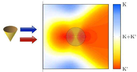
Figure 2: Valley occupation of electrons incident from the left. The shaded area shows the bubble position. Incident current has equal components of K and K' electrons (blue and red). The current is filtered by the nanobubble such that only the K' electrons (red color) are present after passing the bubble.
