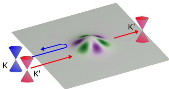
Figure 1: Electrons in K and K' valley impinging on a graphene nanobubble with a strain induced pseudomagnetic field, as indicated by the green and purple colormap. Electrons in valley K are backscattered by the pseudomagnetic field distribution while the electrons in valley K' are transmitted.
