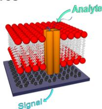
**Fig. 1:** Electrochemical biosensor with supported protein/lipid membrane.
