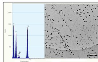
**Fig. 3:** EDX spectrum (left) and TEM image (right) of graphene on nickel TEM grid
