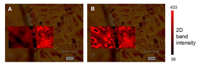
Raman images, superimposed on while light microscope images, from a small region of a graphenecoated copper sample. Image (B) uses focus tracking, whereas image (A) does not and, as a consequence, loses Raman data from half of the Raman image.
