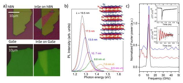
a) Optical images of hBN and GaSe before (left) and after (right) the stamping of a thin InSe nanosheet.b) RT photoluminescence spectra and crystal structure of InSe nanosheets.
