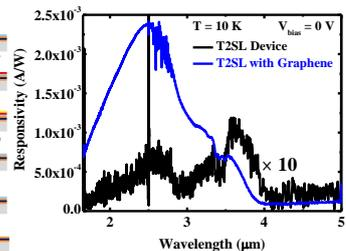
Fig. 4 T2SL infrared photodetectors with and without graphene electrodes.
