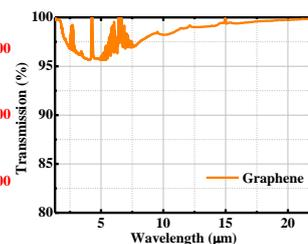
Fig. 2 1.3 - 22.2  $\mu\text{m}$  transmittance of graphene.
