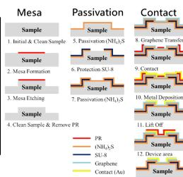
Fig. 3 Device fabrication flow of T2SL infrared photodetectors with graphene electrodes.
