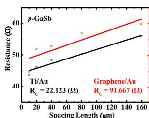
Fig. 1 Resistances of graphene and Au/Ti electrodes with different separations.
