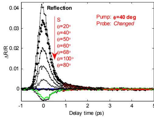
Figure 2. Probe polarization dependence of  $\Delta R/R$ , pump beam is with wavelength of 800 nm.
