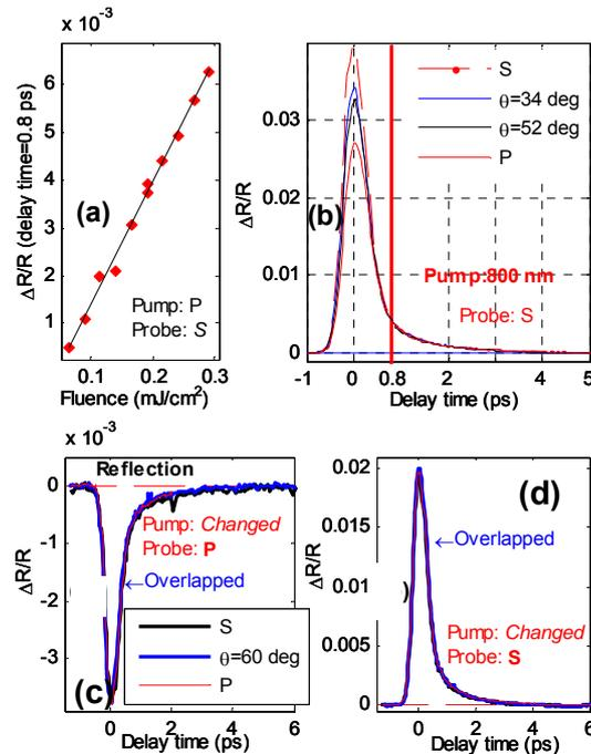
Figure 3. Pump polarization dependence of  $\Delta R/R$ . (a) pump fluence dependence of  $\Delta R/R$  signal at delay time of 0.8 ps. (b) pump polarization dependence of  $\Delta R/R$  time scan curves. (a-b) under 800 nm light excitation. (c-d)  $\Delta R/R$  time scan for different polarized pump beam under 400 nm light excitation.
