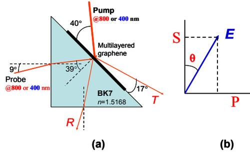
Figure 1. Experimental setups and definition of polarization of beams.
