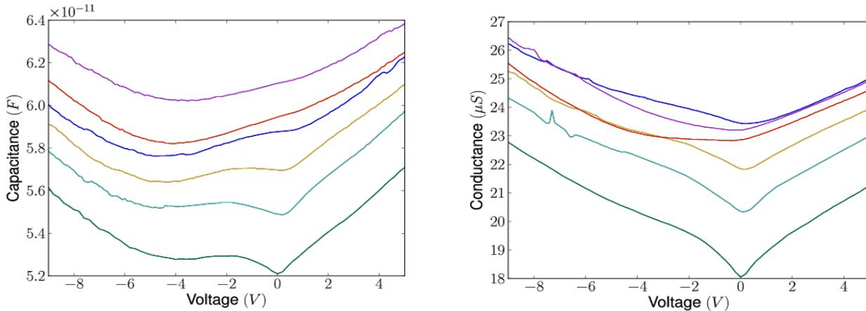
Figure 1 (left): CV measurements taken as a function of temperature from 77 K (green) to 300 K (red). At 77 K a capacitance minimum is observed around 0V indicating the existence of a Dirac Cone. The capacitance is measured on a MOS structure with a circular pad of diameter 400  $\mu m$ .
