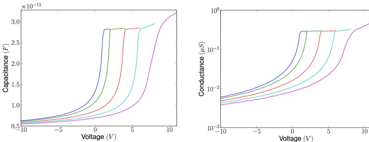
Figure 3 (left): CV measurements on SiC reference samples taken at 77 K. Accumulation is visible near 10 V positive bias. The movement to the right of each successive sweep indicates the filling of deep traps within the Al<sub>2</sub>O<sub>3</sub>. Measurements are taken at 100 kHz.
