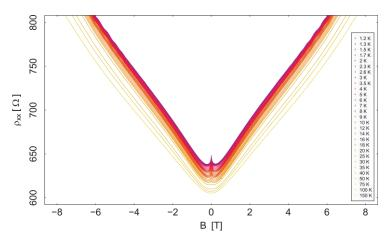
Linear magnetoresistance measured in large area devices of bilayer epitaxial graphene on SiC(0001).
