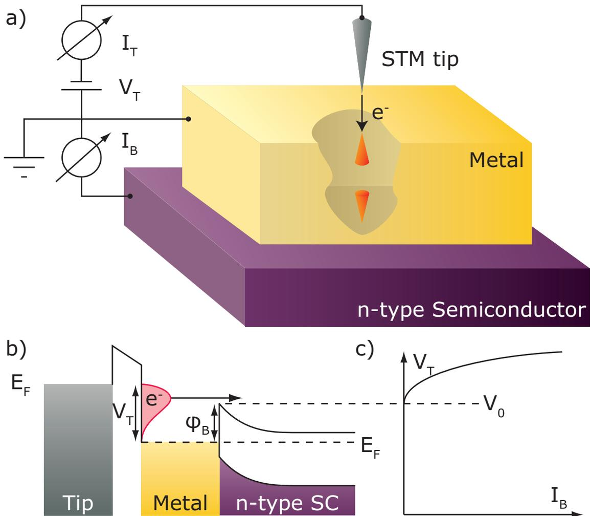
**Figure 1:** a) Schematic representation of BEEM with the electrical connects. b) Energy schematics of the metal-semiconductor device along with the STM tip. The tip is biased negatively and a distribution of hot electrons is injected into the metal. c) The measured BEEM current  $I_B$ , consists of electrons with proper energy and momentum to surpass the Schottky barrier ( $\phi_B$ ), as a function of the tunneling voltage  $V_T$ .
