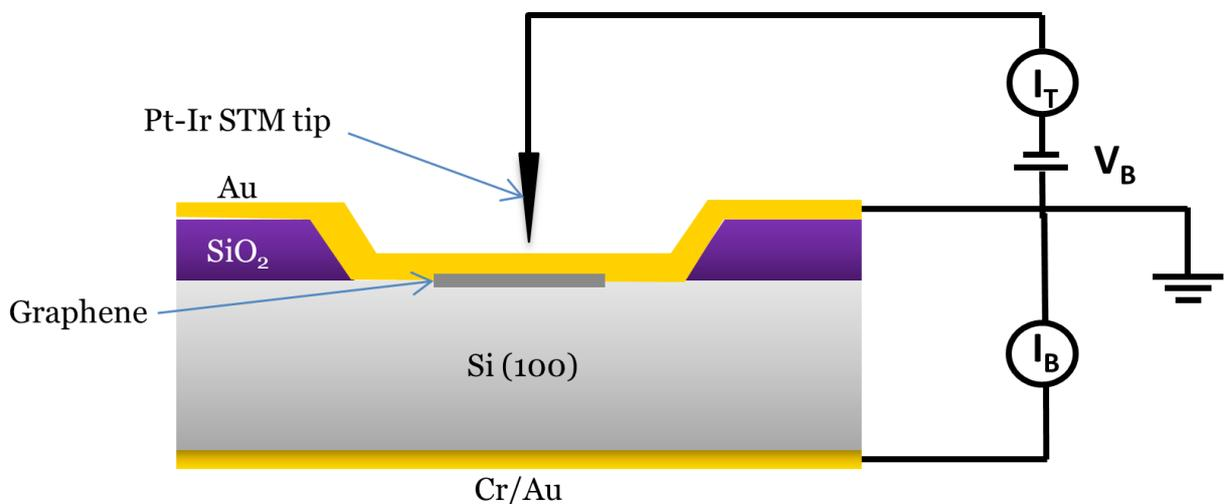
**Figure 2:** Schematic side view of our device scheme. Hot electrons tunnel from the STM tip into the Au from which they travel to the graphene. The transmitted hot electron current at the graphene/Si interface is collected as the BEEM current  $I_B$ .
