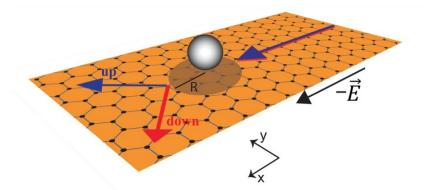
Schematic picture of extrinsic spin Hall effect generated by transport skewness. An impurity (sphere) near the graphene sheet causes a local spin-orbit field with range R. The scattering of components with positive (negative) angular momentum is enhanced (suppressed) for charge carriers with spin up (down), resulting in a net spin Hall current.
