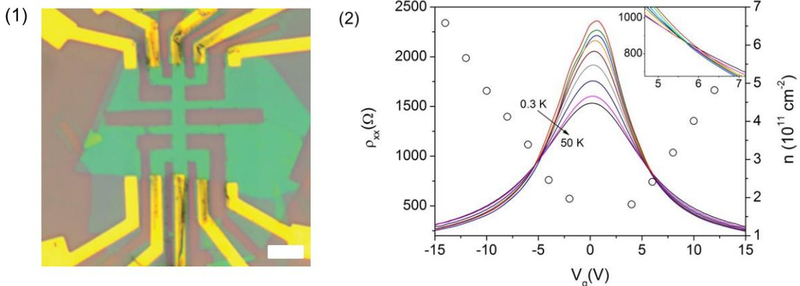
**Fig.1** Optical microscopy image of a bilayer graphene device. The uppermost h-BN flake is clearly visible on top of the graphene/lower-h-BN mesa and the metallic contacts. The scale bar is 5  $\mu\text{m}$ .
