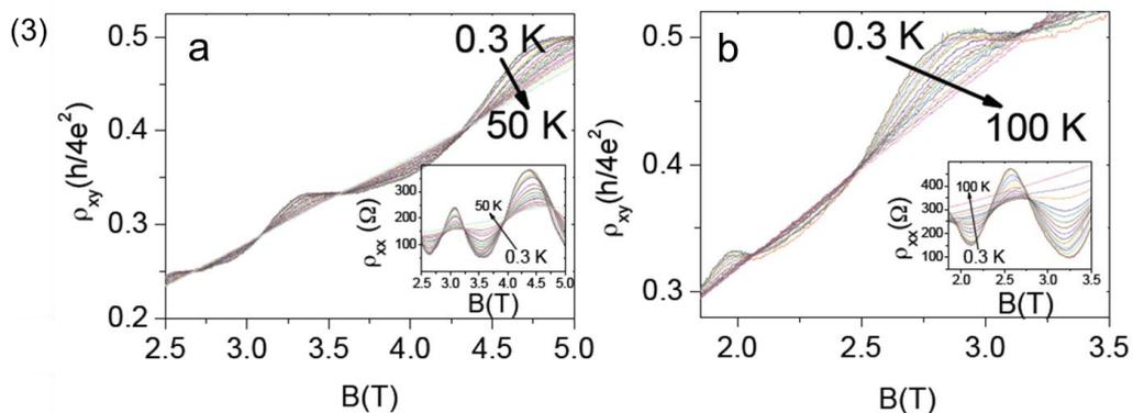
**Fig.3** Panels (a) and (b) show the isotherms of the Hall resistivity  $\rho_{xy}$  as a function of the magnetic field in the electron-like regime at densities  $n = 10.2 \times 10^{11} \text{ cm}^{-2}$  and  $n = 6.1 \times 10^{11} \text{ cm}^{-2}$  respectively. The P-P transitions 8-4 and 12-8 are visible in (a), the 8-4 in (b). The insets show the isotherms the longitudinal resistivity  $\rho_{xx}$  as a function of the magnetic field. Adapted from Ref. 3.
