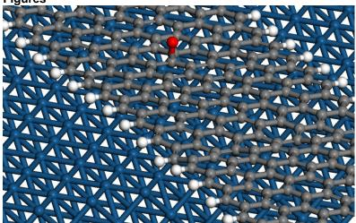
Oxygen adsorption on GNR/Pt(111) surface. Blue, gray, red, and white balls are platinum, carbon, oxygen and hydrogen atoms, respectively.
