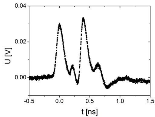
Figure 2: Signal of two FEL pulses with a temporal delay of 500 ps at a wavelength of 42 μm.
