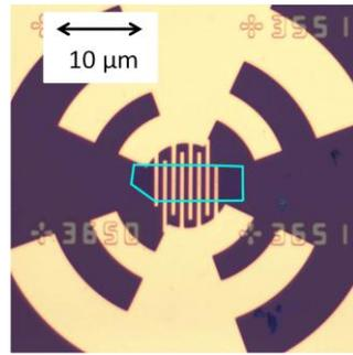
Figure 1: Design of the detector: The graphene flake is in the blue box in the center, the antenna is connected to the flake by an interdigitated structure.
