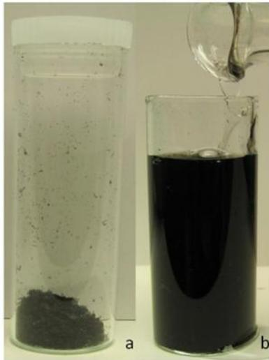
Figure 1: PVP-wrapped graphene may be (a) freeze-dried and (b) readily redispersed, indicating the graphene basal plane is aggregation resistant.
