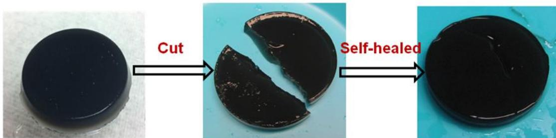
Figure 3: Graphene-loaded polyacrylamide physically-crosslinked gels
