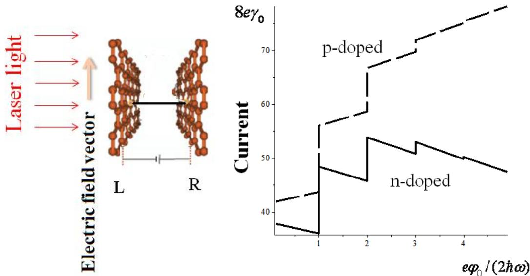
Fig.1. Molecular bridge (thick horizontal line) between left (L) and right (R) graphene electrodes with applied voltage bias. External electromagnetic field acts on the electrodes.
