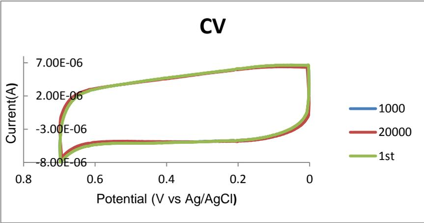
Figure 3 cyclic voltammetry of graphene foam in KCl solution.
