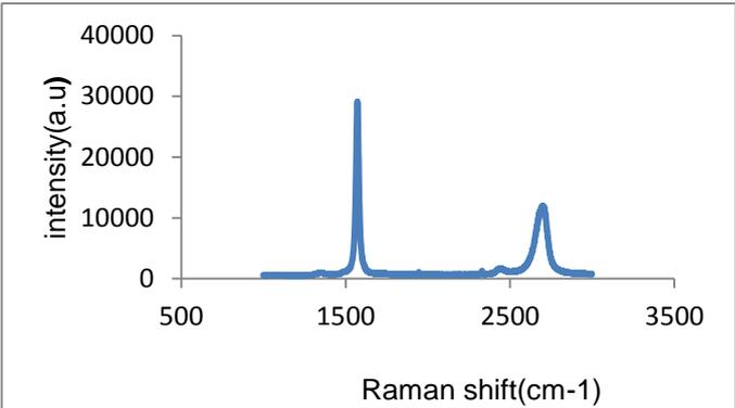
Figure 2 Raman spectroscopy of graphene foam.
