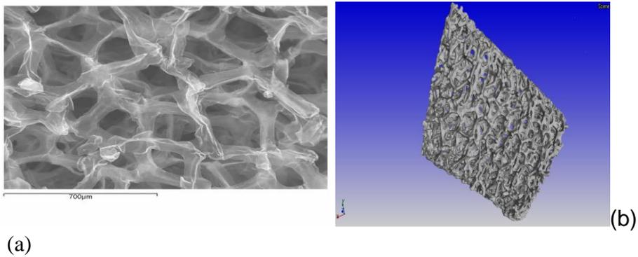
Figure 1: a,b SEM images of graphene foams.
