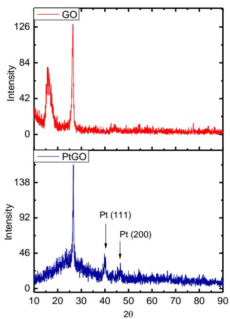
**Figure 2:** XRD spectrum of synthesized Pt/GO nanoparticles
