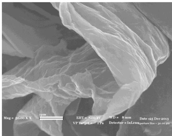
**Figure1:** SEM image of graphene nanosheets
