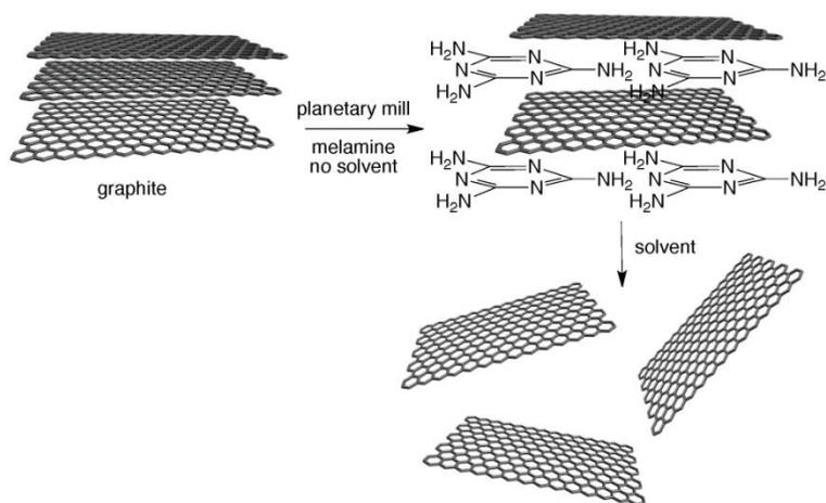
Figure1: Schematic illustration for the exfoliation of graphite through ball-milling approach
