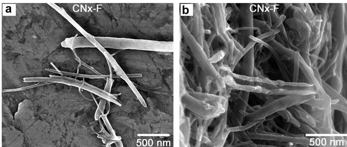
**Figure 1.** SEM images of (a-b) unzipped CNx-MWNTs using the technique involving a mild acid treatment followed by an abrupt thermal shock involving liquid nitrogen and boiling water.
