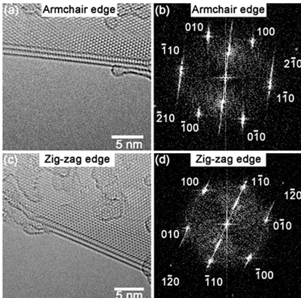
**Figure 2.** (a), (c) HRTEM images and (b),(d) fast Fourier Transformations of the edges of CNx-MWNT nanoribbons with (a,b) armchair and (c,d) zig-zag edges.
