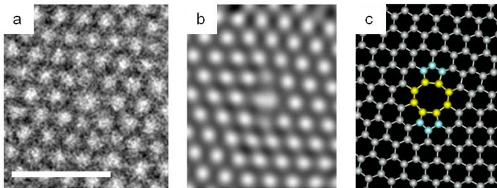
Fig. 1 An example of 5-8-5 defect in graphene. (a) HR-TEM BF image, taken at 120kV. Octagon is almost at center between two pentagons at up and down side (b) simulated TEM image and (c) relaxed atomic model. Octagon with yellow color and pentagon with blue color. Bar = 1nm. JEM 2010F with the CEOS corrector operated at 120kV.
