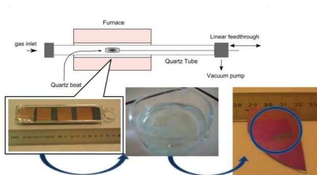
Figure 1 Scheme of the graphene growth apparatus and transfer
