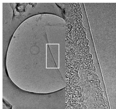
Figure 2. Tem micrograph of single layer graphene film grown in highly diluted methane in hydrogen
