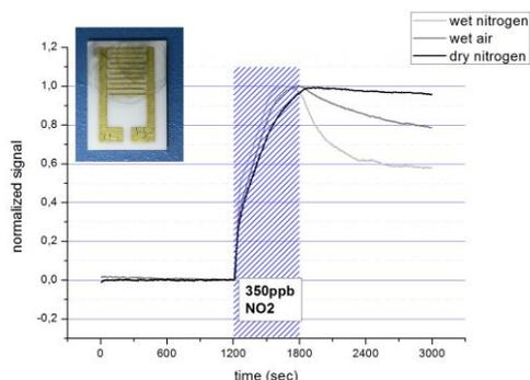
Figure 3: Normalized conductance response  $((S-S_0)/(S_{max} - S_0))$  kinetics upon exposure to 350 ppb of  $NO_2$  in dry and wet carriers, with a flow of 500sccm at 22 °C. The device is DC biased at 1V. In the inset a device photograph of is reported.
