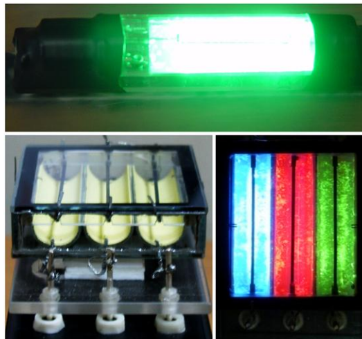
Fig. 2 The photographs of the cathodoluminescent lamps with the nano-graphite cold cathodes accordingly to [3].
