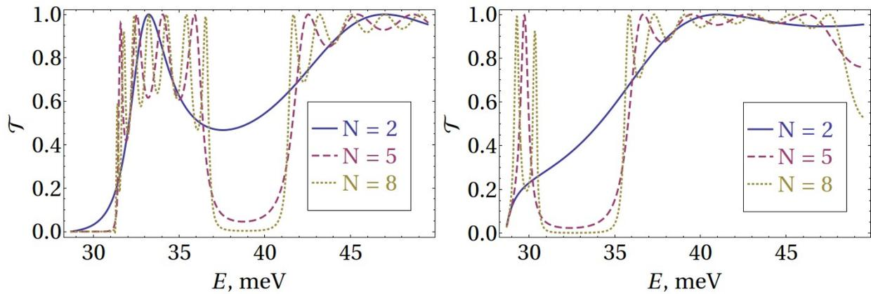
Figure 2: Transmission coefficient as a function of the energy for spin up (left plot) and spin down (right plot) states, for the superlattice described in the text and different number of barriers  $N$ . As  $N$  increases, energy minibands appear, surrounded by regions with vanishing transmission probability.
