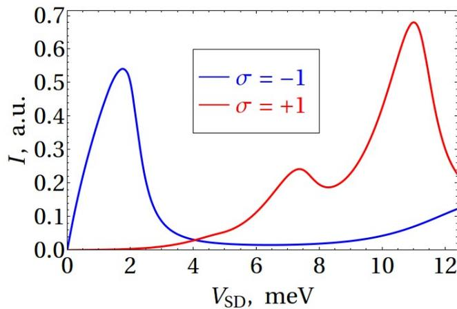
Figure 3: Current-voltage characteristics calculated for  $N = 5$  (at the temperature  $T = 4$  K). Remarkably, the NDR is obtained for both spin states but at different source-drain voltages.
