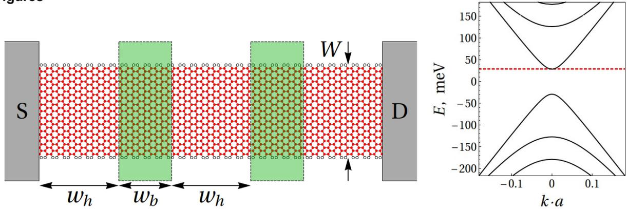
Figure 1: Schematic view of the proposed device (left panel) and the dispersion relation in an infinite aGNR with  $W = 10$  nm (right panel). The dashed line indicates the equilibrium Fermi level at  $\varepsilon_F = 28.5$  meV.
