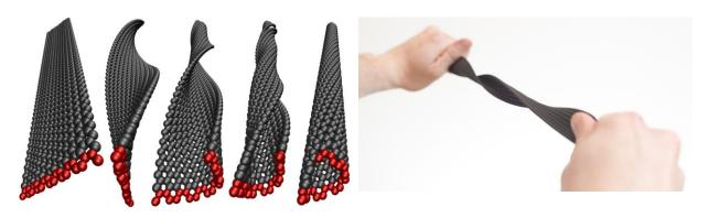
Left: Snapshots from quantum simulation of a 24-Å wide zigzag graphene nanoribbon being twisted into a pristine (9,3) carbon nanotube. Right: The concept of tube formation can be illustrated simply by twisting the ends of a strap of a backpack.
