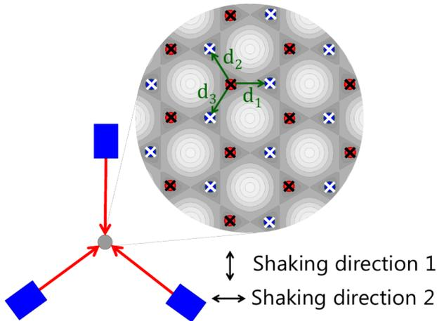
The honeycomb optical lattice is created by three lasers. The two sublattices are indicated by black and white crosses. The vectors joining nearest-neighbor lattice sites and the two studied shaking directions are shown.
